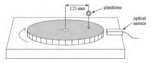
The turntable is made to rotate and then it rotates freely. The lump of plasticine is dropped from a small height above the turntable and sticks to it. Results from the experiment are as follows.
