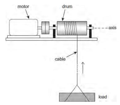
The drum, axle and other rotating parts have a moment of inertia about the axis of rotation of 7.4 kg  $m^2$ , and the mass of the load is 85 kg. The drum has a radius of 0.088 m.
